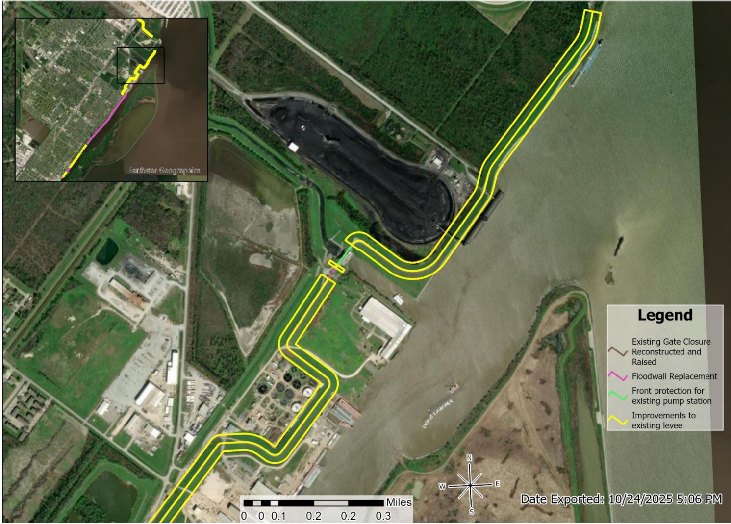
Figure 22 This portion of the project includes the reconstruction of an existing gate structure, floodwall replacement, front protection for an existing pump station and improvements to the levee.
