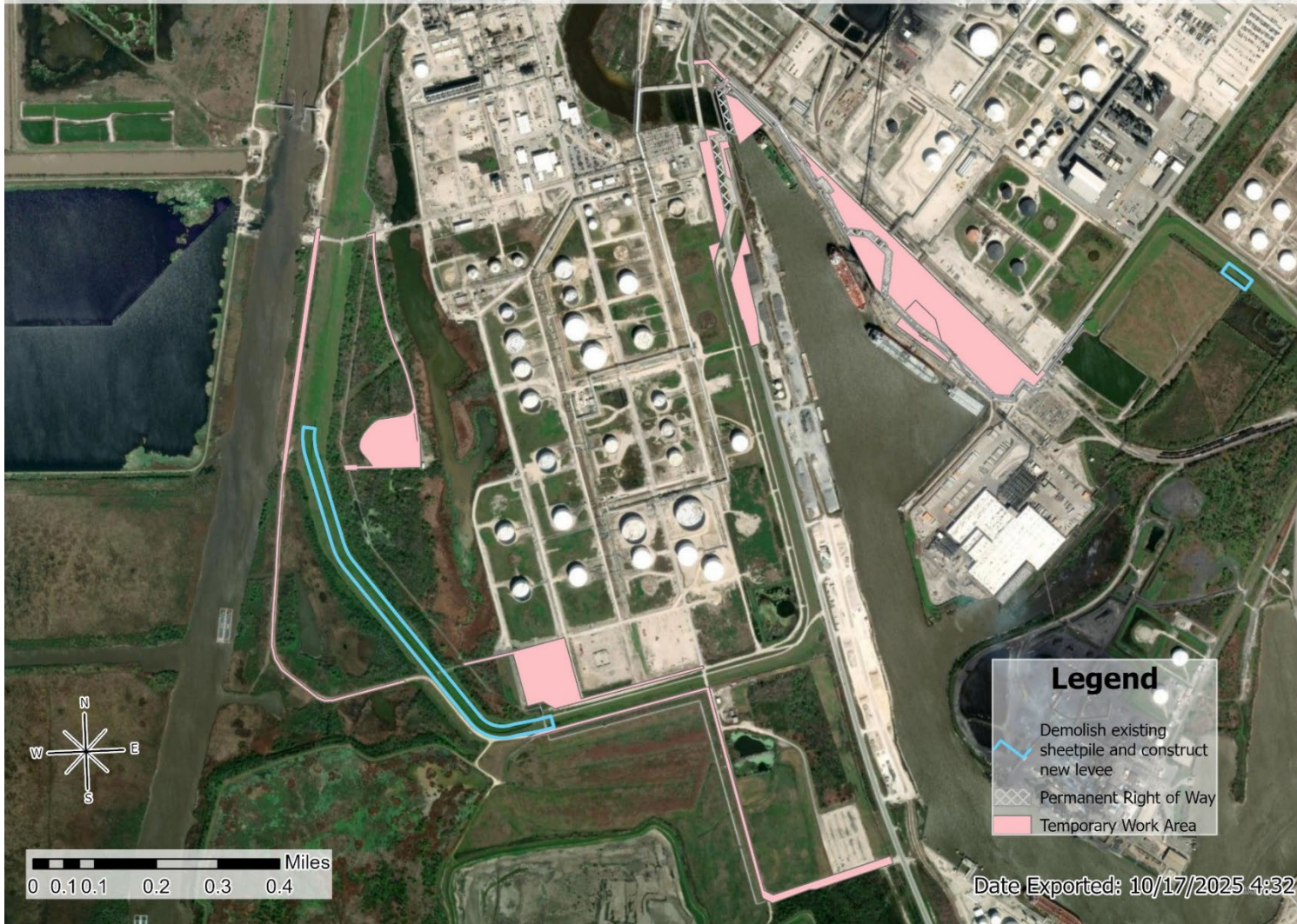
Figure 2 Areas in blue indicate portions of the existing levee system that are currently sheetpile I-wall. Project footprint will expand more significantly in these locations.
