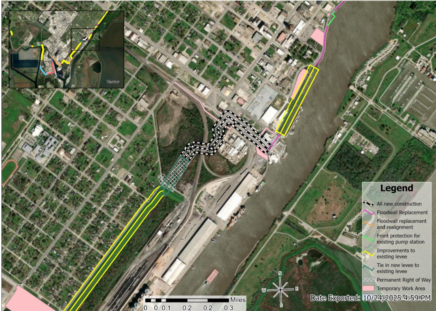
Figure 18 This portion of the project area includes the realignment of the area previously coordinated with the SHPO's office in 2022 as PAV03b. This area includes temporary staging areas and access routes, improvements to existing levee, construction of completely new levee, realignment/replacement of floodwall, and front protection for existing pump stations.
