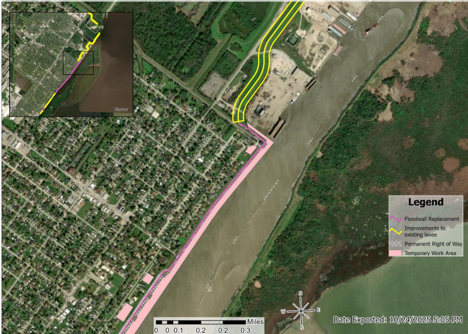
Figure 21 Floodwall construction as described in the previous figure transitions into levee improvements as the project extends to the north.
