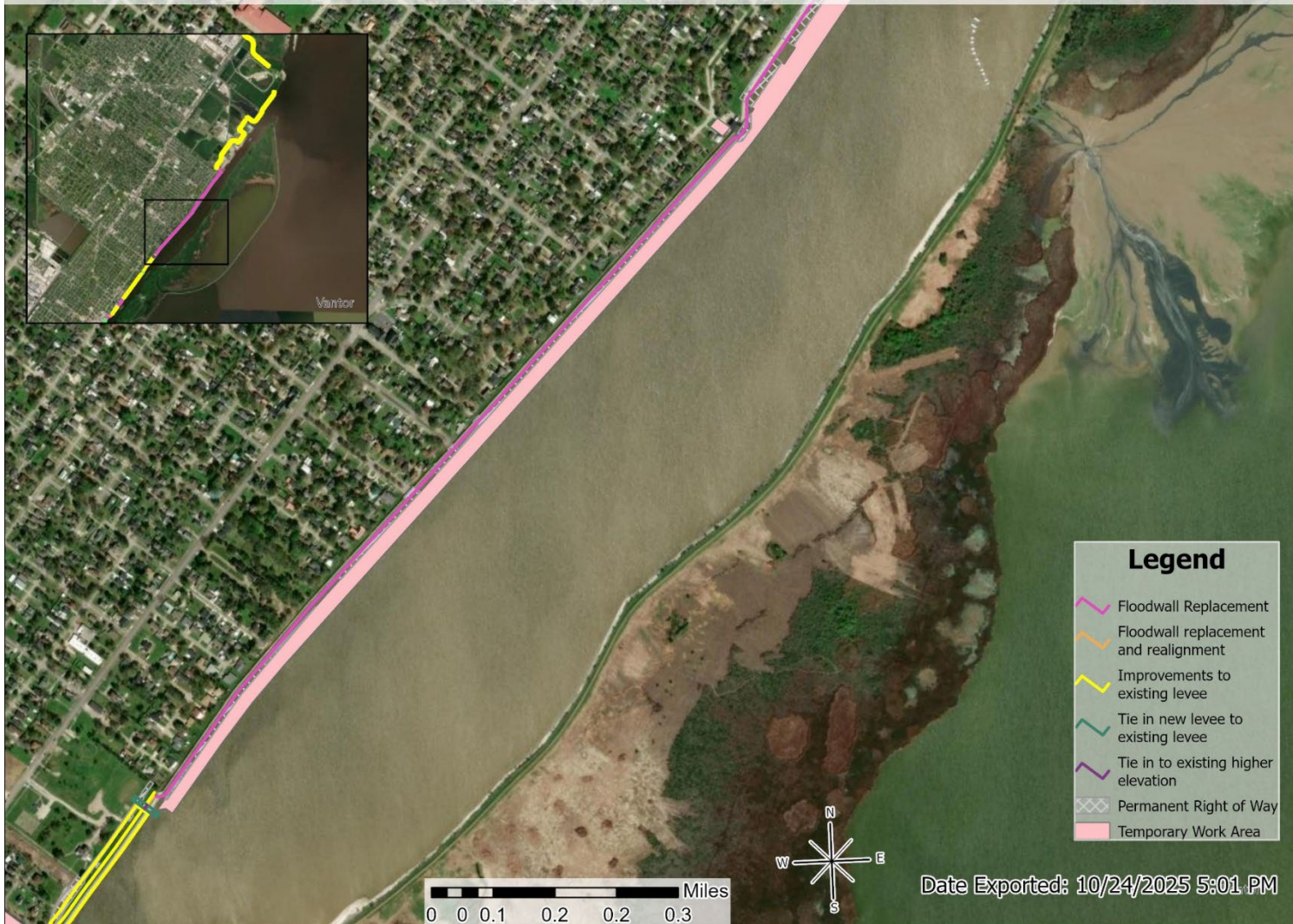
Figure 20 Floodwall to be constructed in the water. Existing floodwall to be demolished. Most of the construction work will be conducted from the water; however, access and staging areas are required landside.
