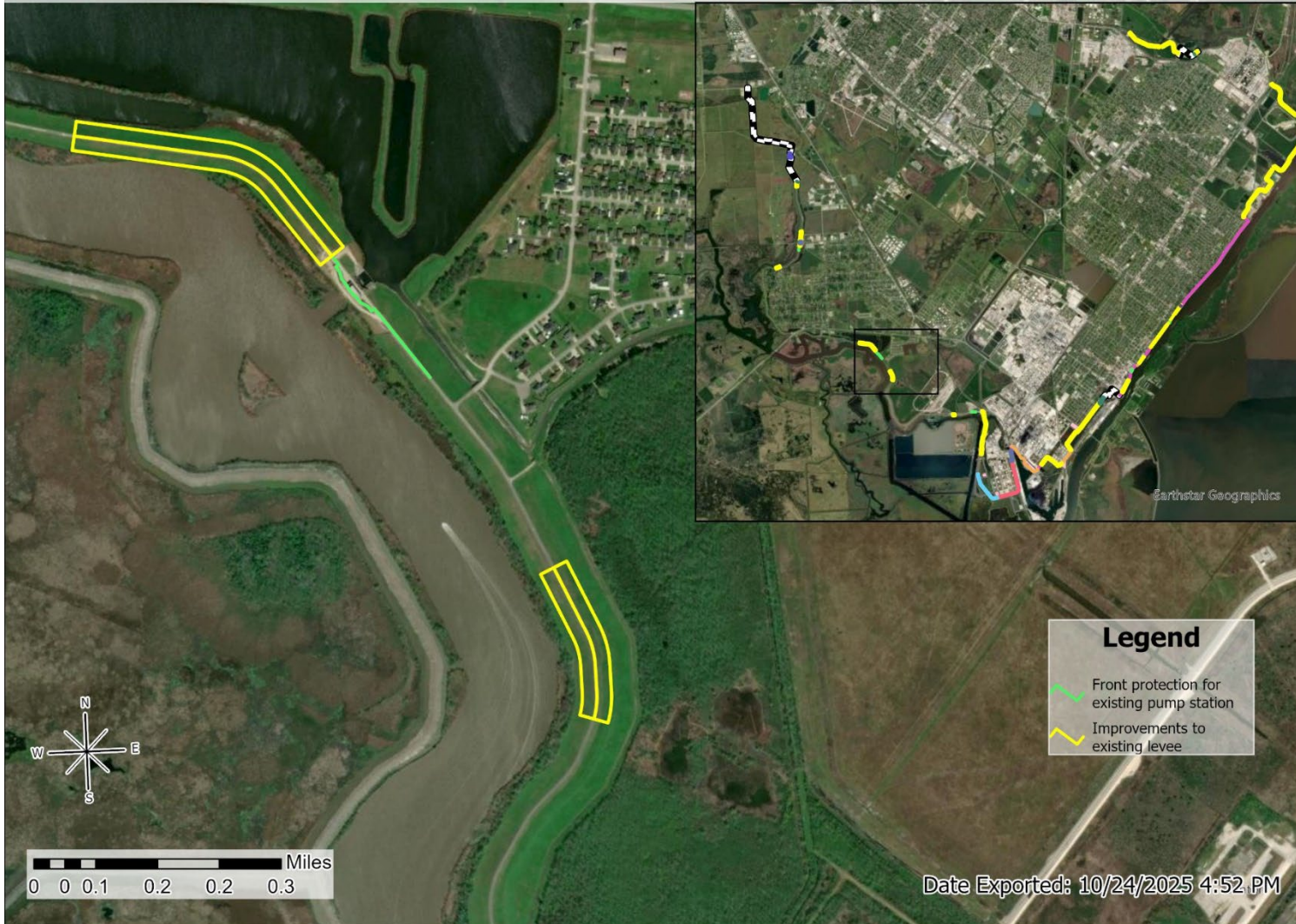
Figure 15 This portion of the project area includes improvements to the existing levee system and construction of new front protection for an existing pump station.
